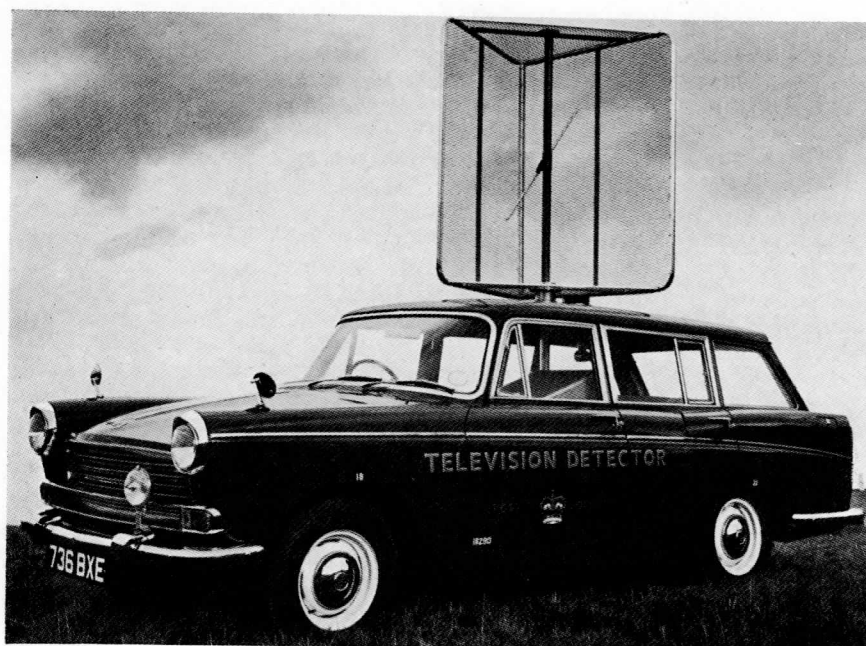
FIG. 1—DETECTOR CAR AND AERIAL
